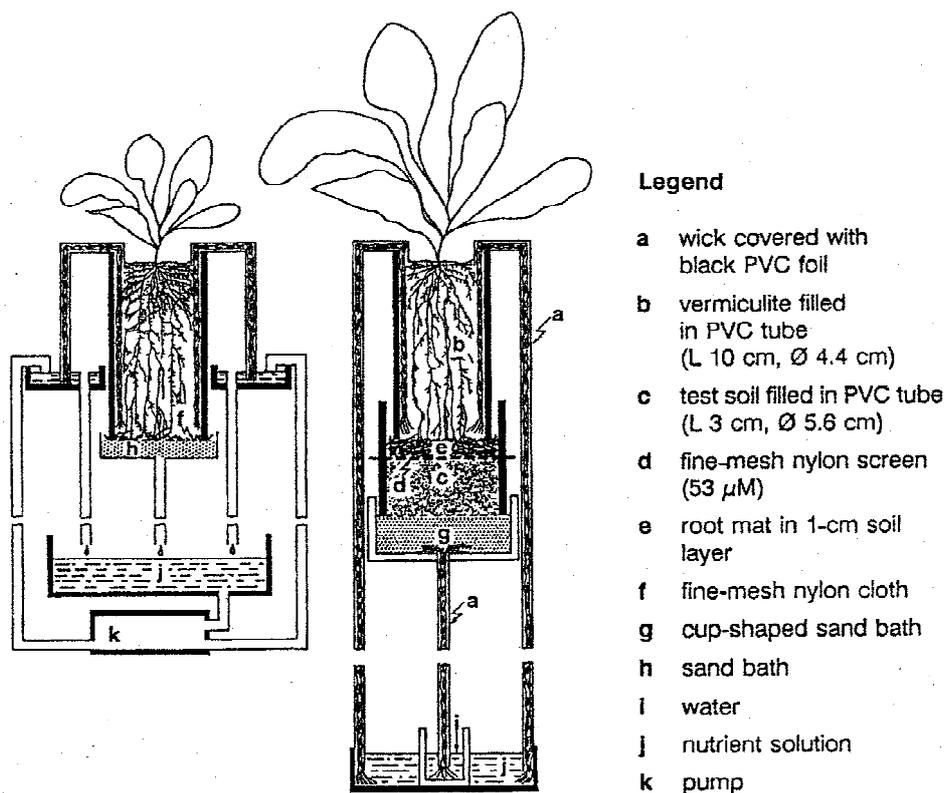
Figure 1. The pre-experimental (left) and experimental (right) set-up according to Gahoonia and Nielsen (1991).
